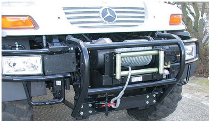
Front bumper mounting on high GVW 4x4 utility vehicles.
