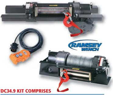
Electric Winch with emergency stop and safety solenoid; load limiting switch; 4.5m heavy duty 2 button wanderlead control; mounting bracket; industrial roller guides with greaseways; 10mm dia. x 30m galvanised wire rope (1960N/mm2 grade) with safety latch hook.
