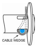
Carefully run winch in the "winch in" direction. Keeping tension on end of cable, spool all the cable onto the cable drum, taking care to form neatly wrapped layers. Keep hands away from drum and guide rollers. Do not allow rope to slide through hands.
