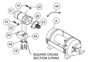
Remove brake housing (No.6) from end bearing (No.4) by unscrewing x 6 cap screws (No.14) in a criss-cross pattern (2 turns each) until all cap screws are removed from brake housing. Remove brake parts from brake housing. Examine brake discs (No.26) for signs of wear, and replace if necessary. Examine O-rings (Nos.34 & 35) and backup rings (Nos.36 & 37) for signs of wear. Remove O-rings and backup rings from grooves in brake piston (No.3). Remove and examine springs (Nos.42 & 43) for damage,
