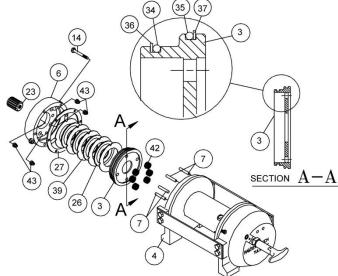
Press larger diameter end of x 4 springs (No.43) into pockets in brake housing (No.6). Place gasket (No.27) on top of end bearing (No.4). Place brake housing over brake parts with fitting ports downward toward mounting feet.
