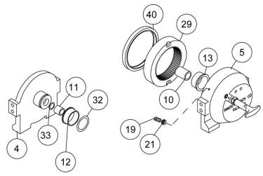
bearing. Install ring gear and nylon setscrew and nut. Ring gear must be fully seated in gear housing end bearing (No.5) and slot in ring gear must NOT be aligned with clutch shifter hole. Install new seal in gear housing end bearing, with sharp edge of seal outward.
