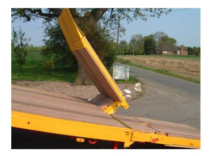
Hydraulic power is required to power the system. This is normally provided by a PTO pump fitted to the vehicle's gearbox which generally is also powering a winch or lorry loader crane which are typically fitted to plant beavertail type bodies. If a PTO pump unit is not fitted, BHW Group Ltd may supply an electro-hydraulic power pack which supplies hydraulic power and is powered from the vehicle's batteries. BHW Group Ltd may also supply PTO pump units if required.
