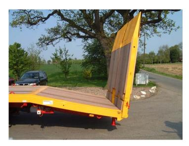
The components supplied include the hydraulic rams, all ramp pivot points and hydraulic ram mounting brackets. The body builder is required to incorporate these components within the build of the ramps.
