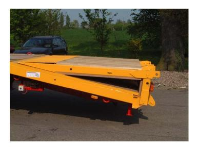
This 'fill in' of the beaver tail results in the flat part of the body being continued fully to the rear. The POWER•WEDGE ramp system may also be operated and stowed as standard loading ramps.
