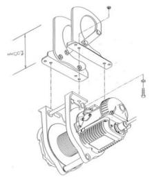
The support bar and its supporting structure must be capable of carrying 125% of the hoist's rated capacity (safe working load), and approved for safe operation.
