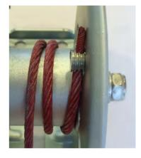
The pictures above show the locking nut and screw supplied with BHW winches to secure the tapered end of the wire rope to the side of the drum.
