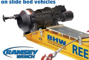
The patented **REEL•SMART**™ system uniquely positions the winch to one side of the slide bed and is able to provide a straight line pull from any angle - even when the connection to the casualty vehicle is offset.
