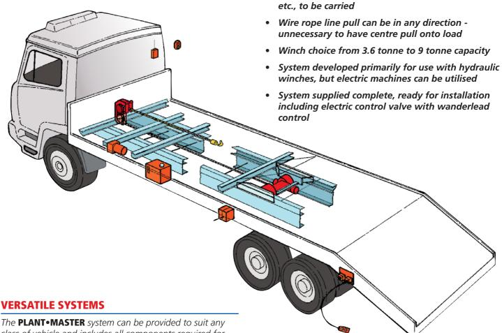
class of vehicle and includes all components required for specific applications.
