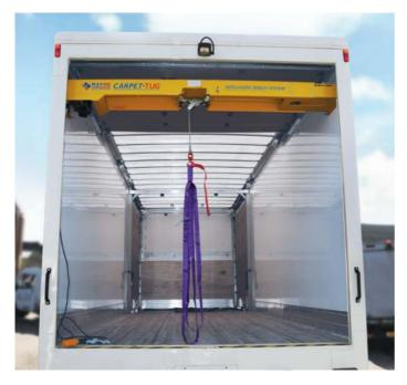
Unloading or reloading with **CARPET•TUG™ 500** is made easy, simply by attaching the wire rope to a webbing harness looped around the end of the carpet roll.
