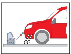
Results in high pull down force on the tow eye and suspension - and strain to the winch as casualty vehicle gets close.
