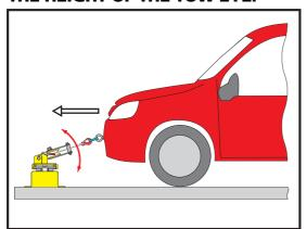
Rotator pivots upwards as casualty vehicle gets close, reducing pull down bending force to nearly zero. The tow eye, the suspension and the winch are all under less strain.
