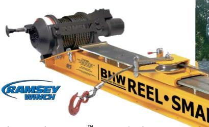
The patented **REEL•SMART**<sup>™</sup> system uniquely positions the winch to one side of the slide bed and is able to provide a straight line pull from any angle even when the connection to the casualty vehicle is offset.
