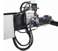
3) Free spool winch drum disengagement / engagement control is normally situated adjacent to the manual operating lever for winch control. This freespool control will disengage the drive from the winch to provide a free running (freespool) drum. NEVER DISENGAGE THE FREESPOOL WITH A LOAD ON THE WIRE ROPE.
