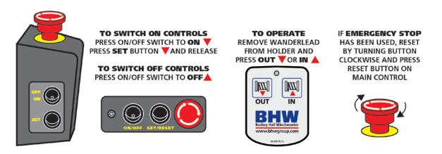
Press the ON/OFF button on the winch control unit once. Press the SET button on the winch control unit.
