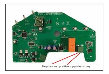
**PLEASE NOTE**. The positive and negative supply from the battery and the red and black cables to the winch must have a minimum of 2.5mm and a maximum of 4mm cross section to avoid any voltage drop. A minimum of 8v through the system must be maintained. The positive and negative terminals on the winch PCB are shown above.
