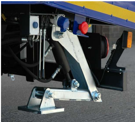
Stabiliser leg in raised position (folded up)
