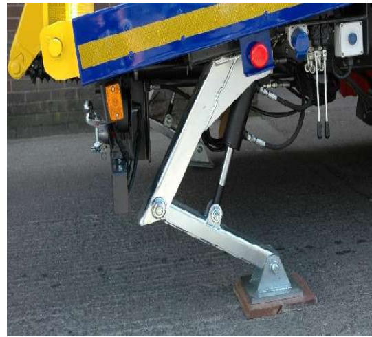
Stabiliser leg fully deployed (folded down)
